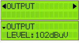
Define the OUTPUT LEVEL of the output signal, selectable between 89-112 dB $\mu$ V (per 1 dB $\mu$ V) and two isolated levels ideal for optical systems: 70 and 83 dB $\mu$ V.
