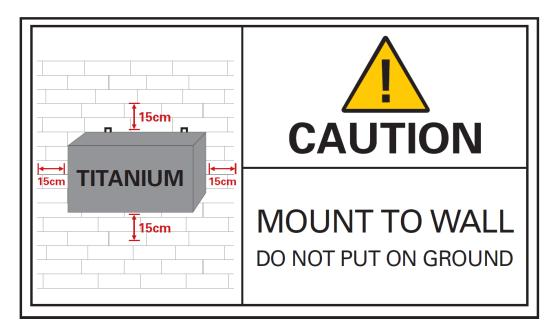
Proper installation is critical to system performance. It is particularly important to install the Titanium correctly in order to receive and distribute optimal signal quality.
