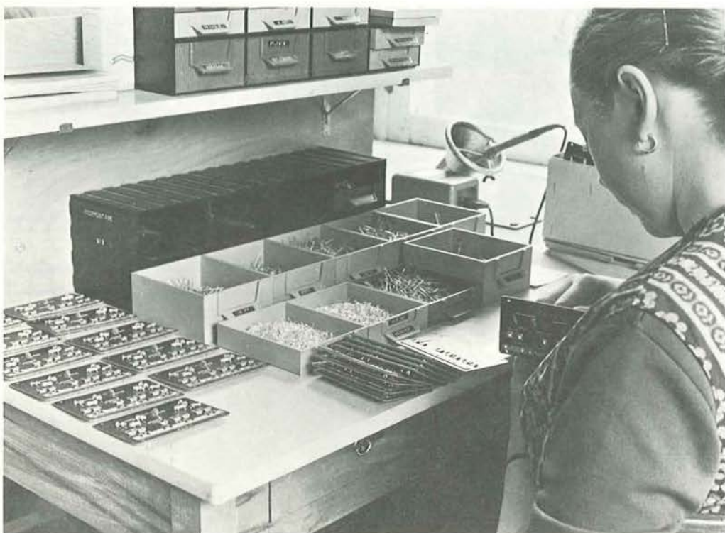
Vóórmontage W13 verbindingsfilters.
