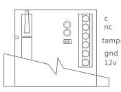
nc 12V: Anode of DC power tamper GN D:Cathode of DC power TAMPER:Anti-tamper switch output NC/C:relay output
