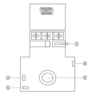
1.Temper Switch4.Lock/Unlock Jumper2.Optional Sensitivity Jumper5.Learning Jumper3.Sensor
