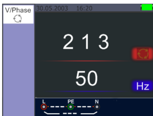
Phase Sequence – When connected in counter-clockwise manner
